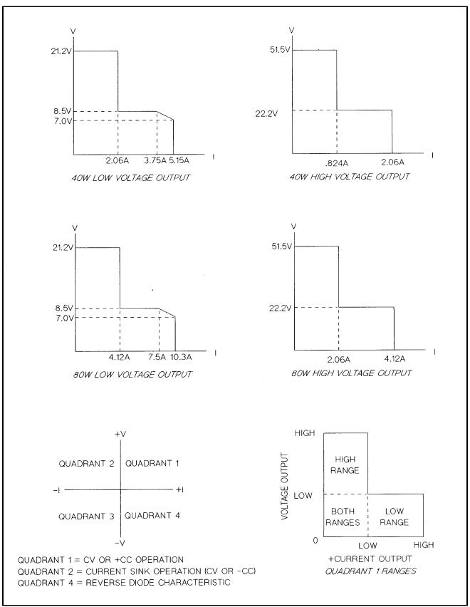
Figure 4-2. Typical Output Range Characteristics
